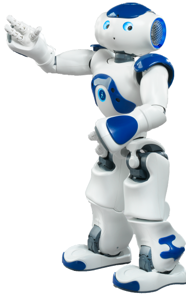
Figure 3.1.: The robot Nao from Aldebaran Robotics.
